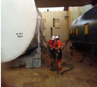
Securing the heavy turbine 290 tons
