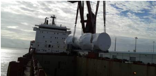
Lifting 290 tons turbine. In tandem ship's crane operated by ship crew.
